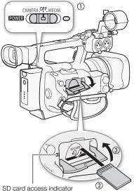
• SD cards have front and back sides that are not interchangeable. Inserting an SD card facing the wrong direction can cause a malfunction of the camcorder. Be sure to insert the SD card as described in step 3.
