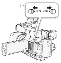
2 Insert the CF card straight, with the label facing away from the lens, all the way into the slot until it clicks (②).
